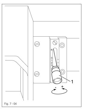
• Adjust the stitch length by turning the knurled nut **1** accordingly.
